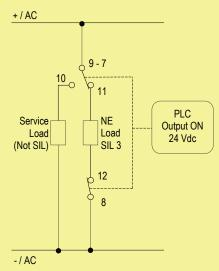
Contacts 7-11 and 8-12: in normal operation relays are energized, contacts are closed, NE load is energized.
