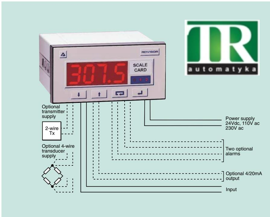
The **Advisor A75** is a universal panel meter for displaying process variables in engineering units. In addition to the features offered by the fixed range A70, the A75 has twelve on-site selectable process voltage and current inputs. The meter is housed in a robust enclosure with high quality push-buttons, display and terminals and will provide many years of reliable service.
