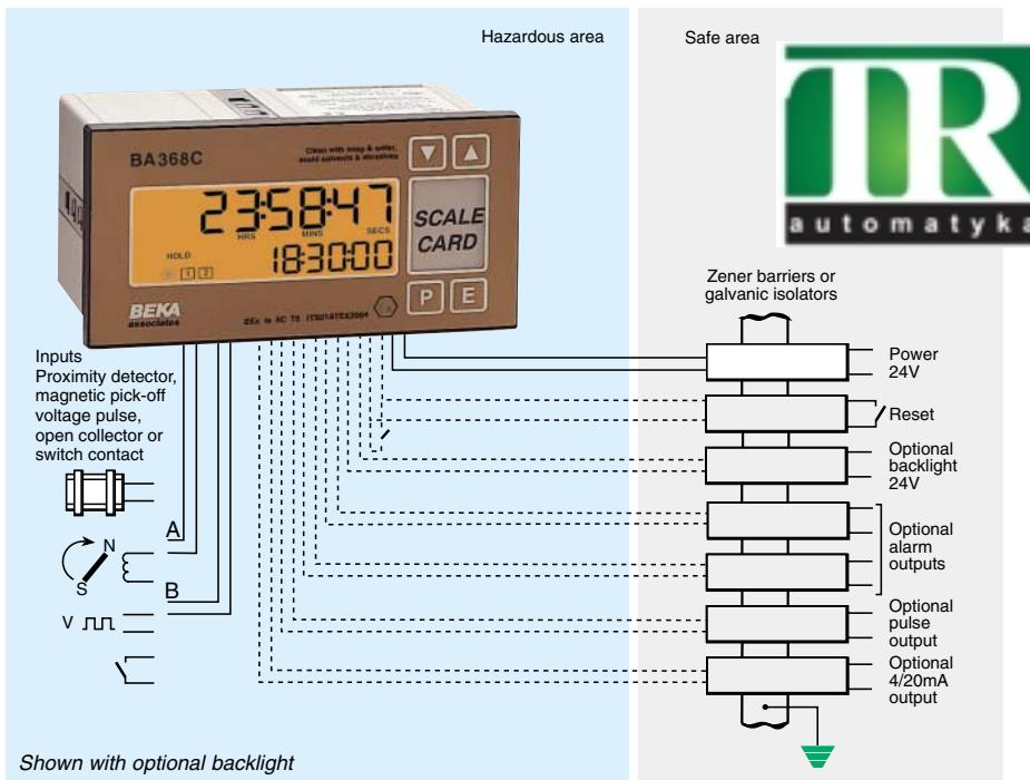
**The BA368C** is an intrinsically safe multi-function instrument which may be programmed to perform a host of counting and timing functions. Easy to use menus allow the instrument to be configured as a counter, timer, tachometer or as a clock. Both of the inputs will operate from 2-wire proximity detectors, switch contacts, magnetic pick-offs, open collector or voltage pulses. Optional alarm/control outputs further extend the many applications.
