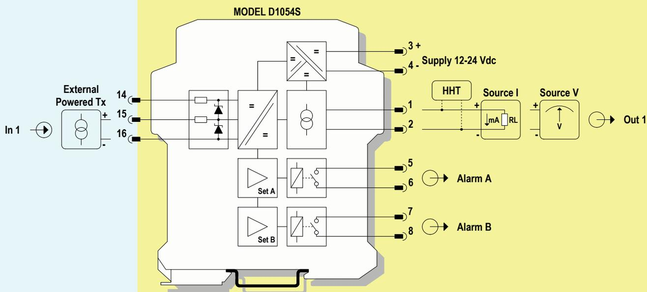
**For SIL applications, alarm contacts must be used in series with equal configuration. Relay contacts shown in de-energized position.**
