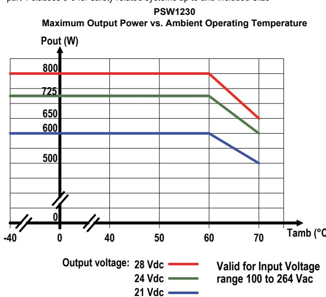
With 50% redundant configuration (two PSW1230 with paralleled outputs), each module can give 350 W power output up to 70°C operating ambient temperature, with output voltage range 21-28 Vdc and input voltage range 100-264 Vac.
