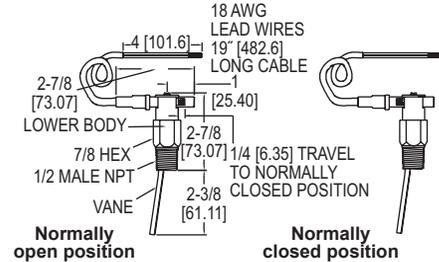
The **Series V10 FloTECT® Mini-Size Flow Switch** is designed to provide inexpensive, reliable monitoring of the presence or absence of flow in a system. This series is available for field installation in pipelines from 1/2 to 2" diameter and available in brass or 303 SS body.
