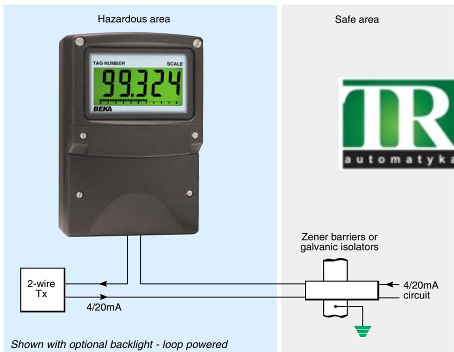
The **BA324E loop powered 4/20mA indicator** is a fourth generation field mounting instrument that is electrically and mechanically compatible with the earlier BA324D. It has a much larger full 5 digit display and guaranteed performance between  $-40$  and  $+70^{\circ}\text{C}$ . Like its predecessor, the BA324E is housed in a robust IP66 enclosure with a separate terminal compartment.
