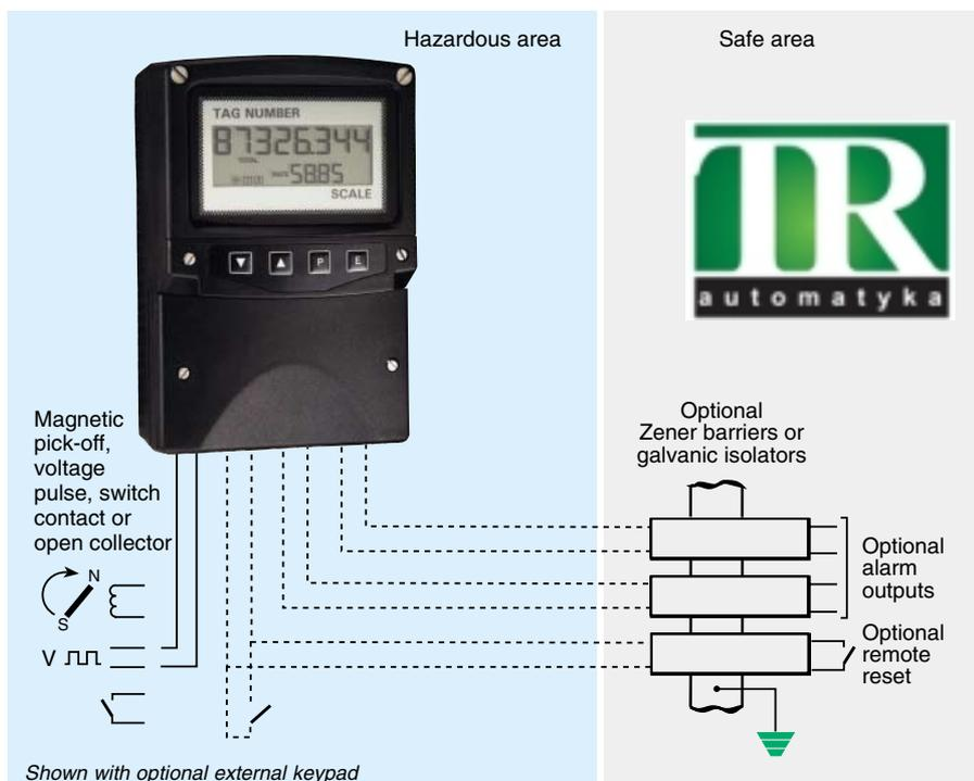
The BA344D is a battery powered, intrinsically safe, rate totaliser with separate rate and total displays. An accumulated grand total may also be displayed. The instrument will count switch contact closures, open collector, voltage pulses and the low level output from magnetic pick-offs.
