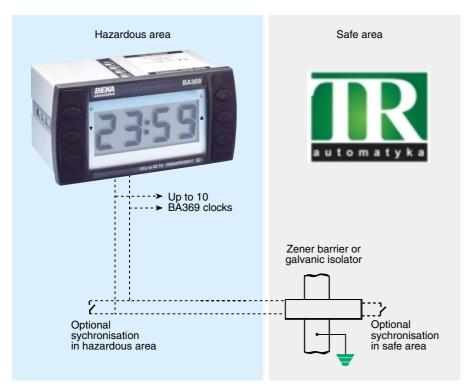
The BA369 is an intrinsically safe, battery powered, panel mounting digital clock that will accurately display local time in a hazardous area.
