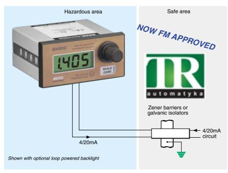
**The BA405C** is an intrinsically safe panel mounting manual set point station that enables the current flowing in a 4/20mA loop to be manually adjusted from within a hazardous area. The instrument is loop powered and contains a  $3\frac{1}{2}$  digit display which may be calibrated to show the 4/20mA current in engineering units.
