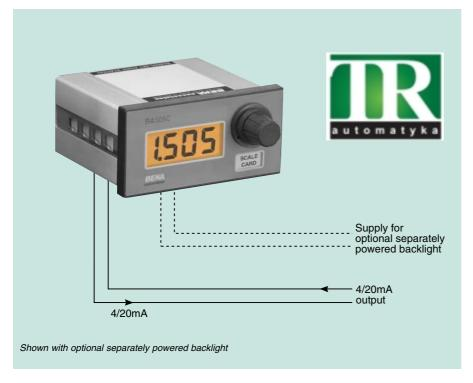
**The BA505C** is a panel mounting manual set point station that enables the current flowing in a 4/20mA loop to be manually adjusted from within a process area. The instrument is loop powered and contains a  $3\frac{1}{2}$  digit display which may be calibrated to show the 4/20mA current in engineering units.
